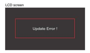
In this case, please contact to support group since the camera might be defective. \* If the SD/SDHC memory card is not Write-Protected, the camera writes out to UPDLOG.TXT file, which file is NG when error occurred.
