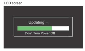
(4) When updating is completed, "Complete" message is appeared on the LCD screen (It takes about 3 minutes for updating) Both slot A LED and slot B LED blinks slowly and simultaneously.
